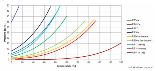
Figure 4 - Refrigerant characteristics: temperature versus pressure
