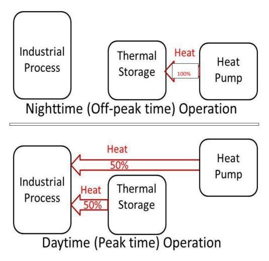
Figure 23 –Heat pump with thermal storage tank
