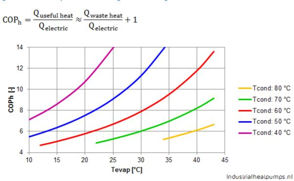
The efficiency of a heat pump, COPh, depends on several factors, especially the temperature difference between waste heat source and potential heat requirement (?). The temperature difference between condensation and evaporation temperature largely determines the efficiency: the smaller the difference, the higher the COPh. The figure above shows the influence of this temperature difference on the COPh value. These values are based on figures from a compressor using Ammonia refrigerant.
