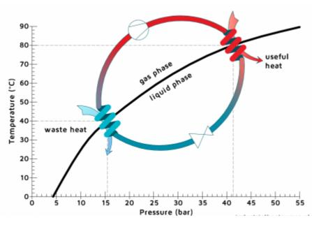
Figure 3 – The thermodynamic cycle (using ammonia)
