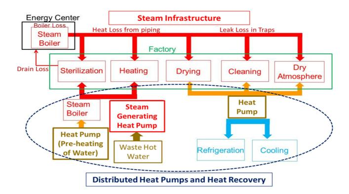
This diagram shows how a series of local heat pumps (in the bottom half of the diagram) can be used to displace an entire boiler and steam system including all the traditional infrastructure (top quarter of the diagram) in a food processing plant. (Note that in this case the steam boiler pre-heated by the heat pump seems was a booster for the small load left to supply a legacy process still needing high temperature steam).
