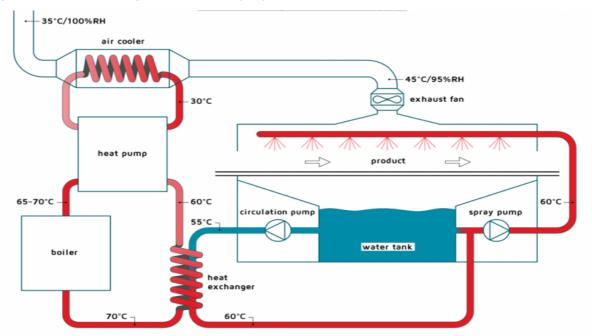
Figure 13 - Industrial washing machine with heat pump
